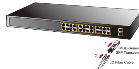
Figure 5-3: Plug In the SFP Transceiver
