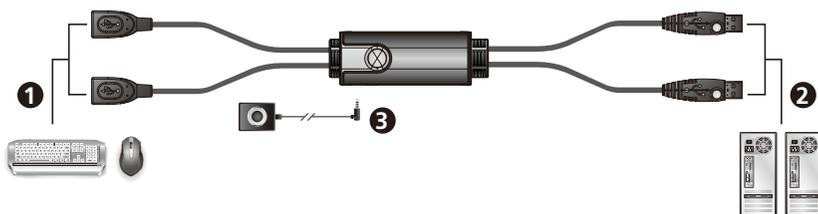
1. Plug your keyboard into the connector at the end of the Keyboard Cable, and plug your mouse into the connector at the end of the Mouse Cable.
