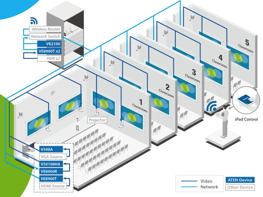
Five classrooms with identical installations connect via the ATEN Video over IP system to enable a matrix of content distribution when there are high numbers of students.
