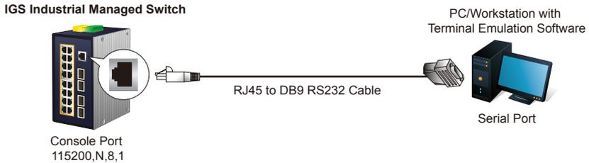
A terminal program is required to make the software connected to the Industrial Managed Switch.
