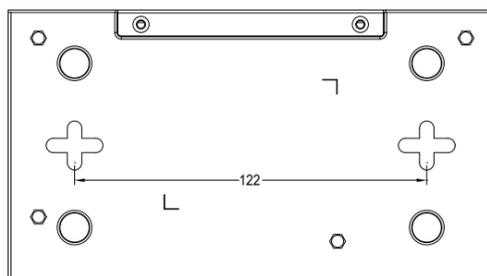
**Step 3:** Hang the GSD-504UP on the screws from the wall.
