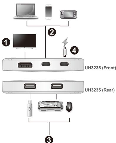
1. Plug an HDMI monitor to the HDMI Output Port of the unit.
