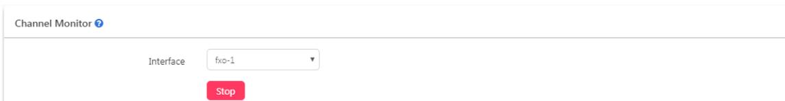
Once the process started the button will change to Stop. Now you should recur the problem by making a call in through the selected interface. When the extension started to ring the third time you may hangup and stop channel monitor by clicking on **Stop** button. As soon as the channel monitor stopped, the captured signaling will be automatically downloaded.
