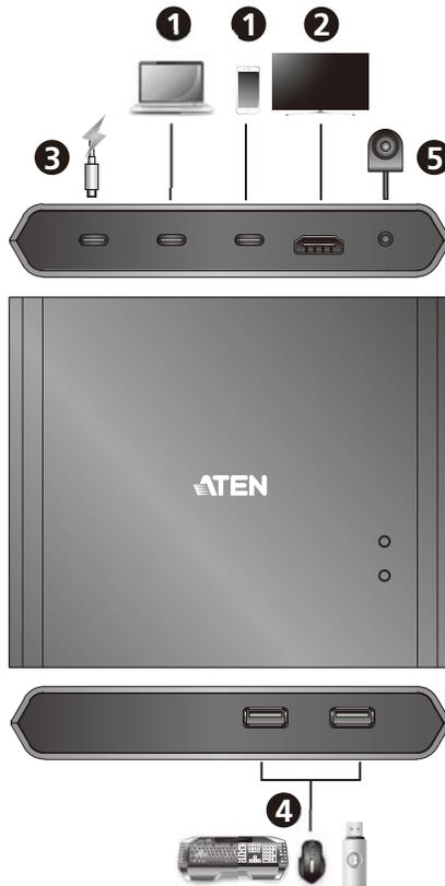
1. Plug the USB-C Cable between your computer and/or mobile device into the back of the US3310.
