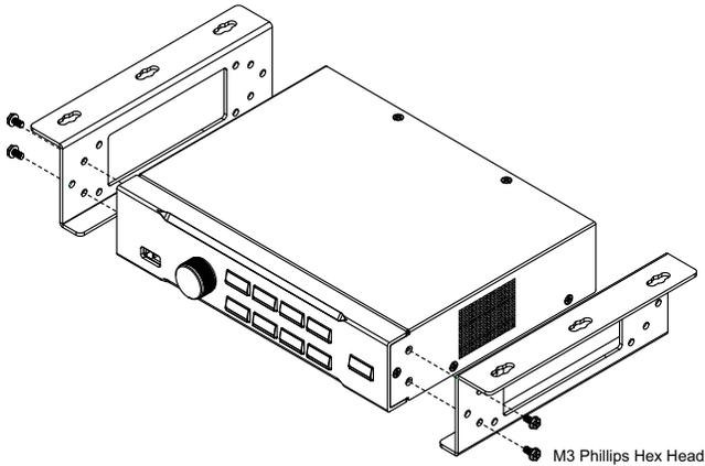
2. Position the unit to a spot under the desk where you can easily access the front-panel pushbuttons, and then secure the racks to the desk with self-prepared screws.
