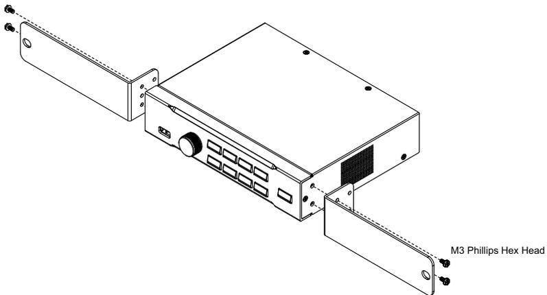
2. Position the unit in the front of the rack and align the holes in the mounting brackets with the holes in the rack.
