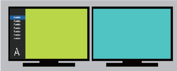
You can also have the connected displays automatically showing identical content using the Mirror Mode feature, which allows display B to automatically follow the source and display settings configured for display A:
