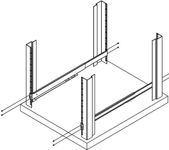
2. Slide the unit along the brackets, then screw the front panel to the rack.
