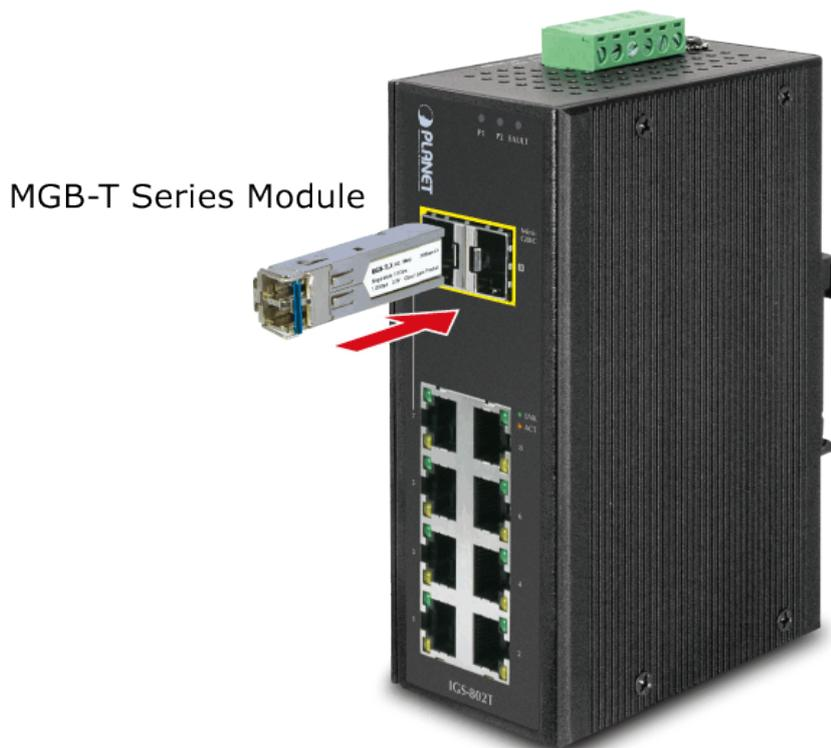
Figure 2-2-4a: Plug in the SFP Transceiver
