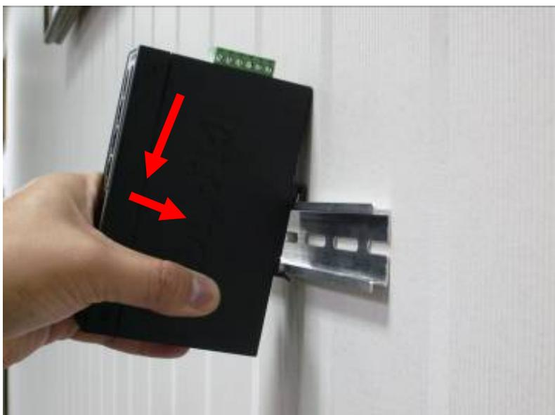
**Step 3:** Check whether the DIN rail is tightly on the track.
