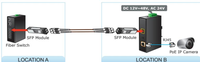
**Figure 2-5:** IGTP-805AT 100/1000BASE-X Installation
