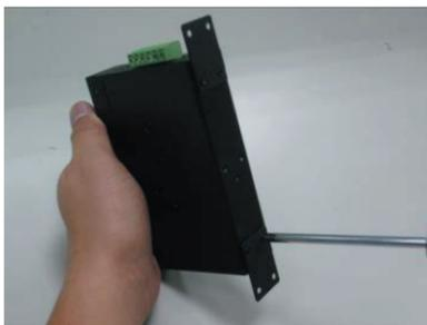
**Step 3:** Use the screws to screw the wall-mount plate on the Industrial 802.3at PoE Media Converter.
