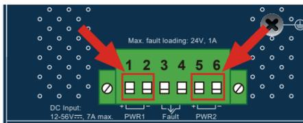
Figure 3-4: Industrial PoE+ Switch DC Input
