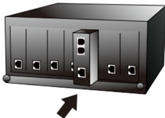
Insert a VDSL2 Bridge into an available slot
