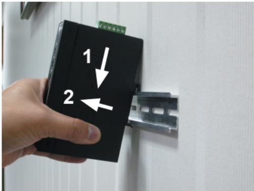
**Step 4:** To remove Industrial Media Converter from the track, lightly lift it up.
