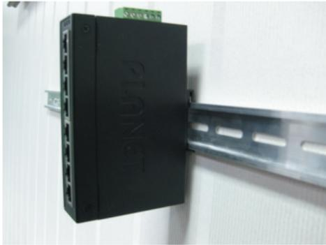
**Step 3:** Make sure the DIN-rail is tightly on the track.
