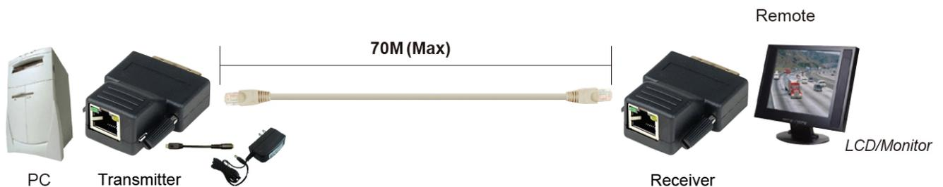
DS-54101 Rev 1-0 transmitter built in micro USB for external power when your DVI source not able to provide enough power to the receiver. For example, when using multiple DS-54101 Rev 1-0 with DVI distributor, the power consumption may over the limitation of the DVI device, please use micro USB to DC plug cable (package included) with 5V power adaptor (optional) for external power.
