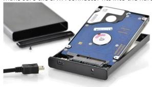
3. Slide the hard disk in and fix the tray by screws in real
