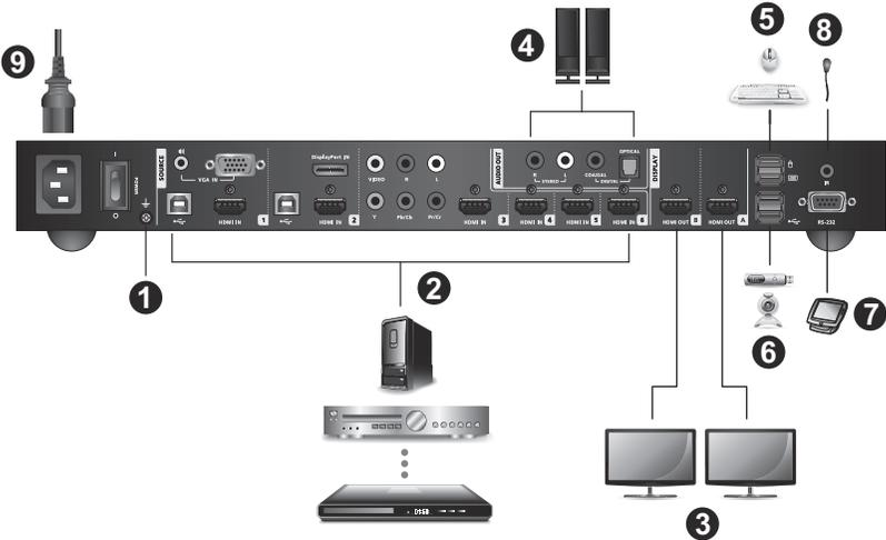
1. Ground the unit with a grounding wire. Connecting one end of the grounding wire to the grounding terminal, and the other end to a suitable grounded object.
