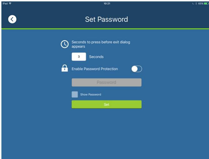
Slide the **Enable Password Protect** button, enter a password in the box and tap **Set**. The *Show Password* option appears after you check enable Password Protect, allowing you to display the characters typed in for the password. Enter a number in *Seconds to press before exit dialog appears* to set the amount of time to pass when pressing on a viewer page before a window appears asking if you want to exit. Tap **Back** to exit.
