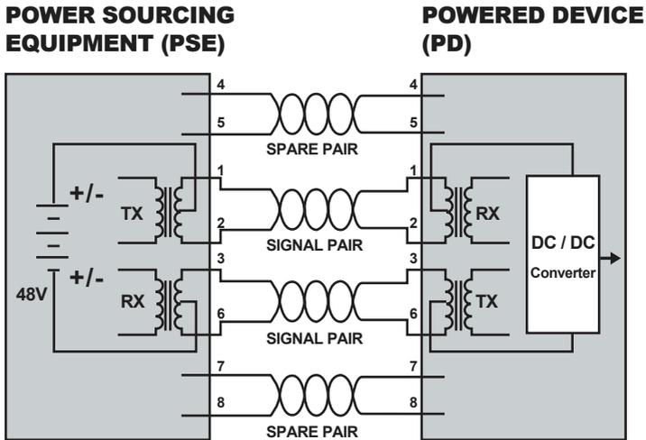
Figure 2: Power Supplied over the Data Pins
