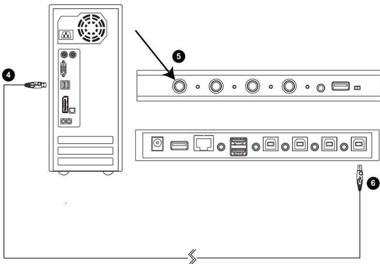
4. Connect the USB Type A connector to a USB Type A port on the computer.
