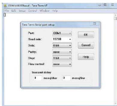
Bits per Second: **19200**, Data Bits: **8**, Parity: **None**, Stop bits: **1**, Flow Control: **None**.
