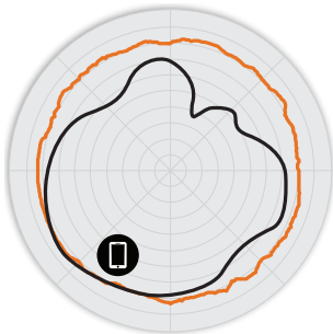
Figure 2. R510 2.4GHz Azimuth Antenna Patterns
