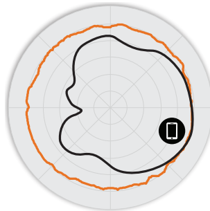
Figure 3. R510 5GHz Azimuth Antenna Patterns
