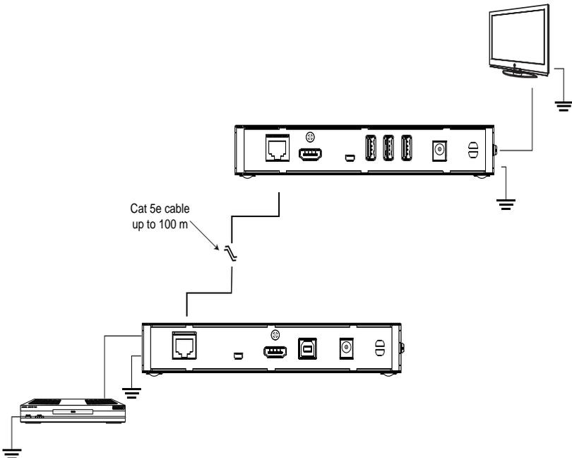
3. For increased grounding protection, use STP (shielded twisted pair) cable to connect the Transmitter and Receiver units. There are two methods that can be used:
