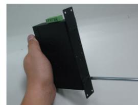
**Step 3:** Use the screws to screw the wall-mount plate on the Industrial Gigabit Ethernet Switch.
