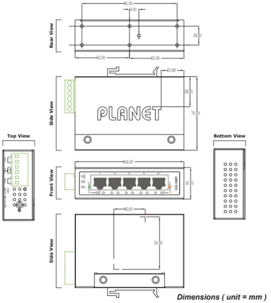
Figure 1: IGS-500T Three-View Diagram
