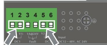
2. Tighten the wire-clamp screws for preventing the wires from loosening.
