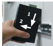
**Step 5:** Lightly pull out the bottom of the switch for removing it from the track.
