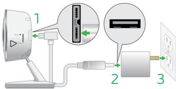
**Ethernet.** Connect the Arlo Q Plus camera to your router with Ethernet, but power the camera with the included micro USB cable and power adapter.
