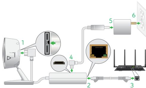
**Power over Ethernet (PoE).** Connect the Arlo Q Plus camera to a PoE switch using the included PoE adapter if you want to power and connect the camera to the Internet with a single cable.
