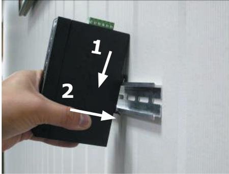
**Step 2:** Lightly insert the bottom of the switch into the track
