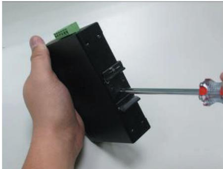
**Step 1:** Screw the DIN-rail on the Industrial Gigabit Ethernet Switch.
