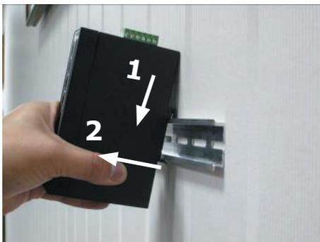
**Step 5:** Lightly pull out the bottom of the switch for removing it from the track.
