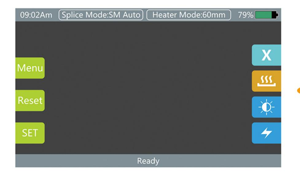
Check the chosen heating mode, press back to return to the initial interface.
