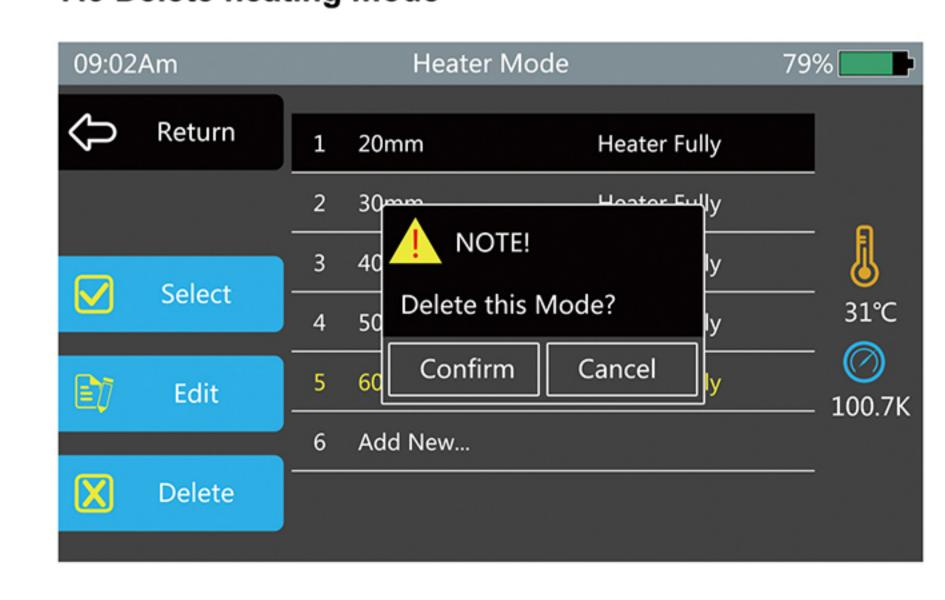
Enter into [Heater Menu], choose the mode you want to delete, press [Delete], press [Confirm] on the tooltip.
