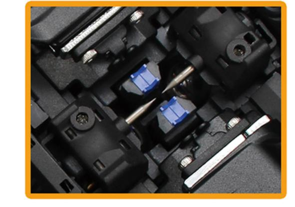
Open heater oven cover Spot of fusion
