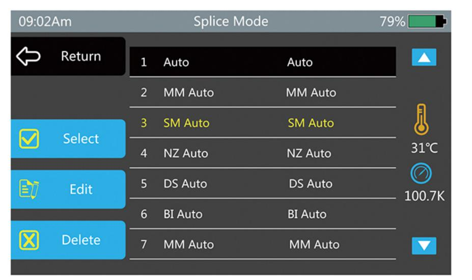
Enter into the splicing mode and select and press the needed one (yellow font is the current splicing mode). Check the chosen splicing mode and press "Return" to return to the initial interface.
