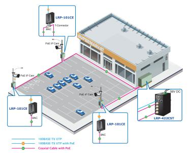
PLANET Long Reach PoE solution provides point to point application for easy plug-n-play operation and deployment in climatically demanding environments with wide temperature range from -20 to 70 degrees C. Without the limit of power source, it makes the installation of remote PoE powered devices easier and more efficiently.
