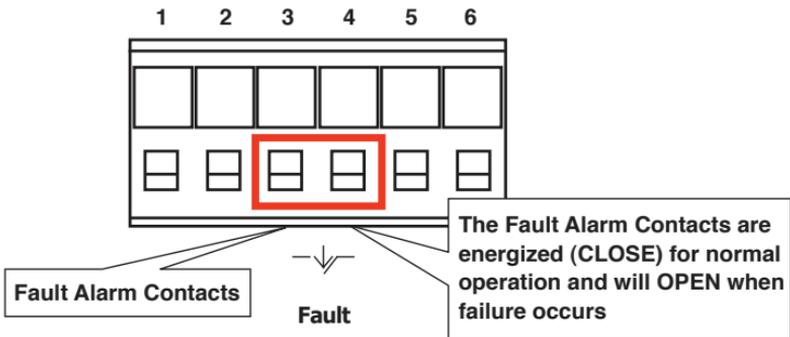
Insert the wires into the fault alarm contacts
