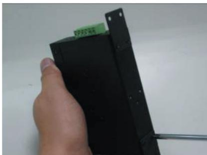
**Step 3:** Use the screws to screw the wall-mount plate on the Industrial Gigabit Media Converter.
