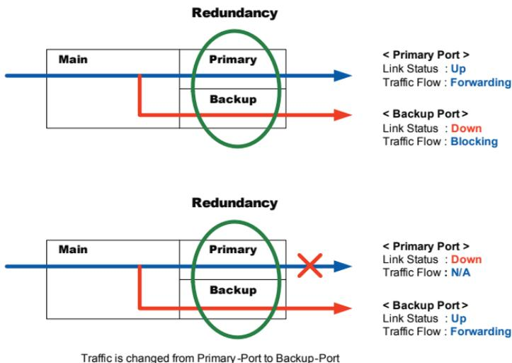
**Figure 3-3:** Redundancy Behavior Topology
