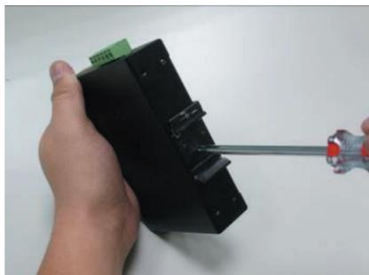
**Step 1:** Screw the DIN-rail on the Industrial Gigabit Media Converter.
