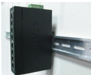
**Step 4:** Please refer to the following procedure to remove the Industrial Ethernet Switch from the track.
