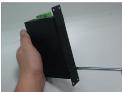
**Step 3:** Use the screws to screw the wall-mount plate on the Industrial Ethernet Switch.
