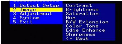
Adjust the picture quality of the display by setting the values for contrast, brightness, sharpness, saturation, hue and sharpness. You can also configure the black and white extension, color tone and edge enhance of your video.
