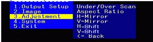
Adjust the picture position on the screen by setting the under/over scan percentage, selecting the aspect ratio and configuring the horizontal and vertical adjustment values.
