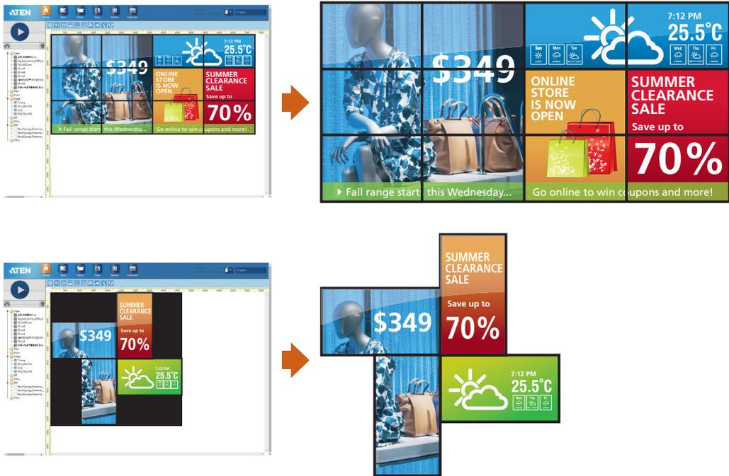
The VS1912 allows you to create asymmetric video wall layouts that can be arranged horizontally and vertically to fit your specific needs. With the flexibility to build a video wall without traditional restrictions, the VS1912 is suitable for a wide range of creative applications in any environment.
