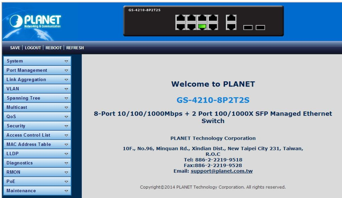
Figure 3-1-4 Web Main Screen of Managed Switch
