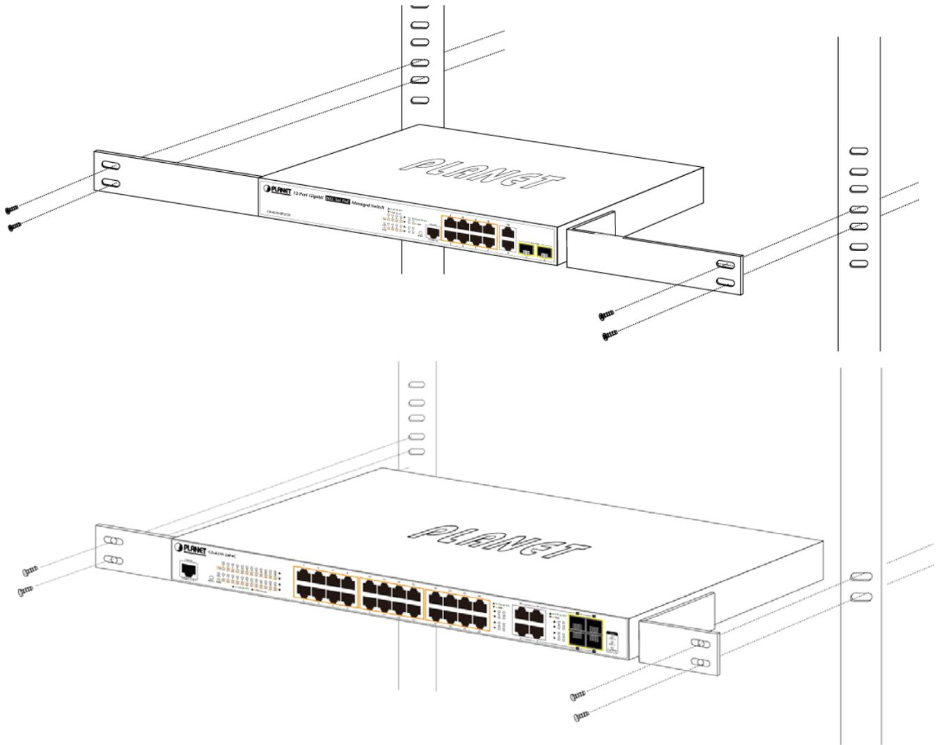
Figure 2-1-6 Mounting Managed Switch in a Rack
