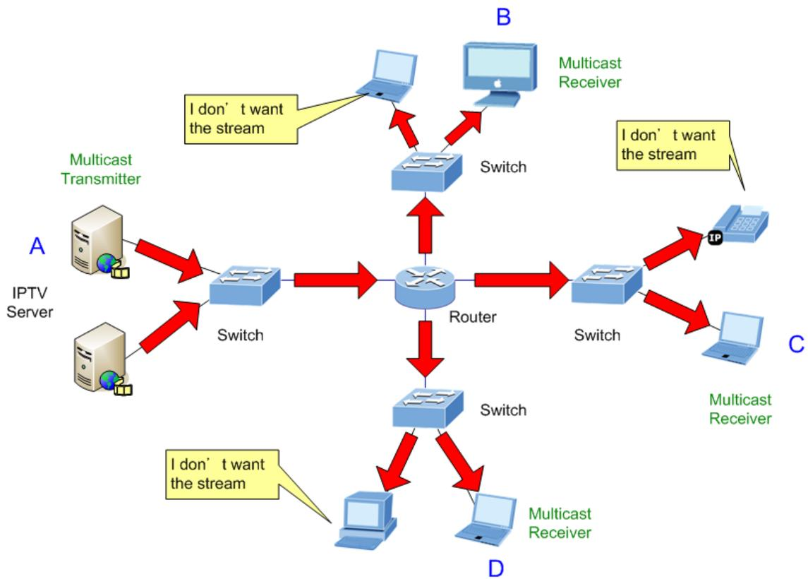
Figure 4-7-4 Multicast Flooding
