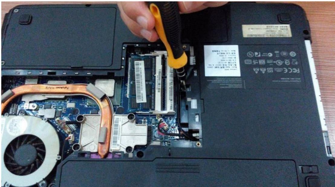
Once remove the CD-ROM driver, please check the thickness of the driver which is 12.7mm or 9.5 mm. In order to pick up the suitable 2nd HDD Caddy, it has to make sure the connector of CD-ROM driver is for SATA or IDE.
