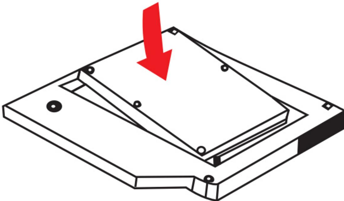
2. Slide the hard drive into the connector until it locks into place.
