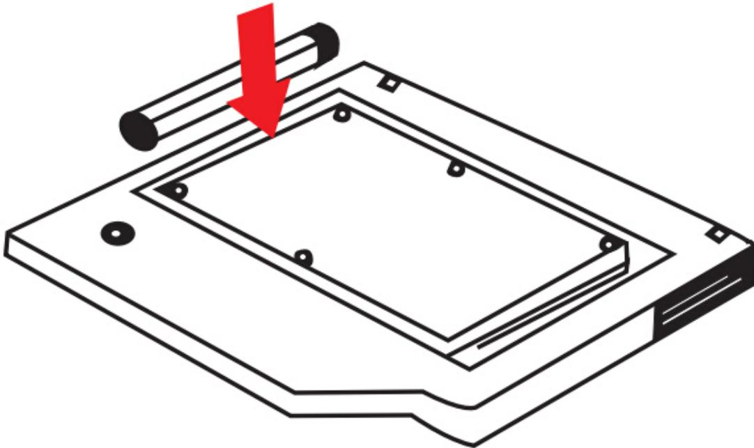
Please assemble the panel and buckle along with the 2nd HDD Caddy, which have been chosen previously.
