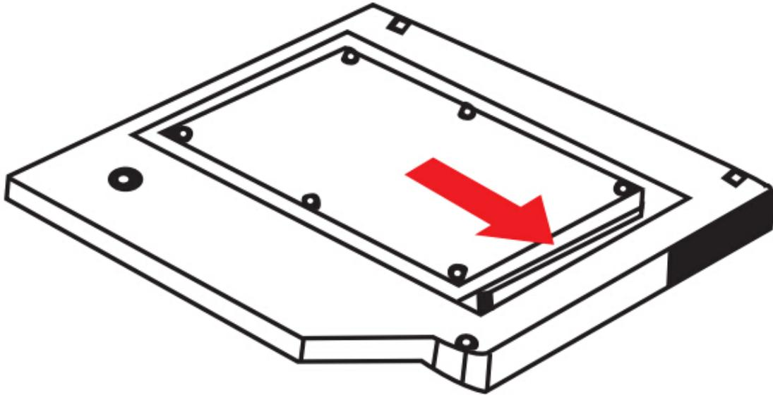
3. Lower the hard drive caddy retaining latch until it snaps closed
