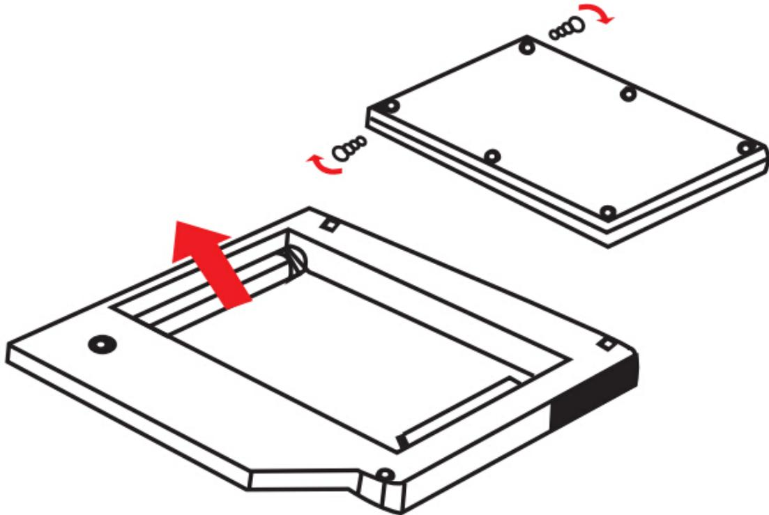
1. Insert the hard drive into the hard drive caddy.
