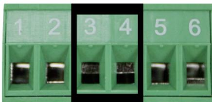
Figure 4: Fault Pin of Terminal Block.
