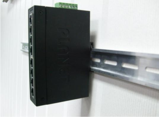
**Figure 7:** Industrial Equipment installed in DIN-Rail mount.
