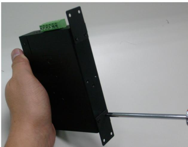
**Figure 9:** Attach Brackets to the Industrial Equipment.
