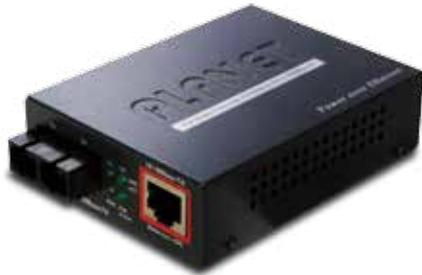
*More than a Fiber Media Converter - a Power over Ethernet Injector as well
