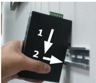
**Step 3:** Make sure if the DIN-Rail is tightly secured on the track.
