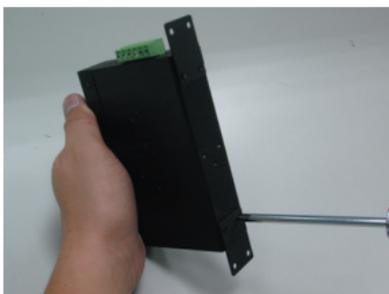
**Step 3:** Use the screws to screw the wallmount plate on the Industrial Gigabit Ethernet Switch.
