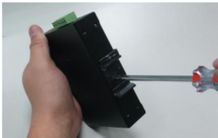
**Step 2:** Lightly insert the bottom of the switch into the track
