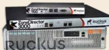
Central wireless LAN controllers supporting from 6 to 1,000 Ruckus APs
