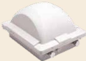
Outdoor dual-band, two-port 802.11n AP with integrated smart antenna array and PoE (802.3af/at) support
