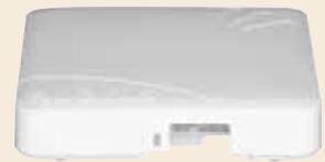
Indoor single-band, two-port 802.11n AP with integrated smart antenna array and PoE (802.3af/at) support
