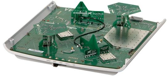
Patented smart antenna arrays in every access point provide longer range and more reliable Wi-Fi connections, requiring fewer APs than competitive alternatives.
