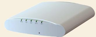
Entry level dual band, 2x2:2 802.11ac AP with integrated smart antenna array and PoE (802.3af) support
