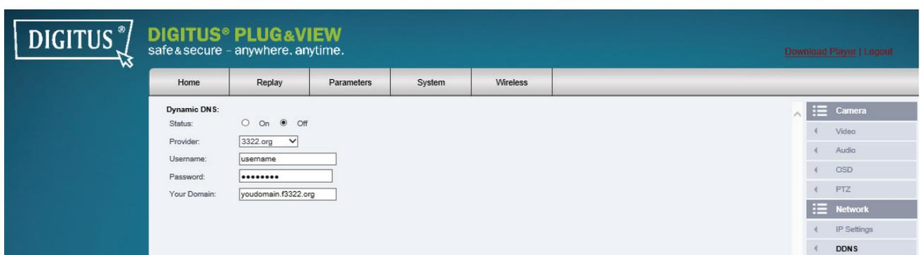
If you want to have additional access to the user interface via a DynDNS provider, activate Dynamic DNS by selecting "on" and enter your domain and access data.
