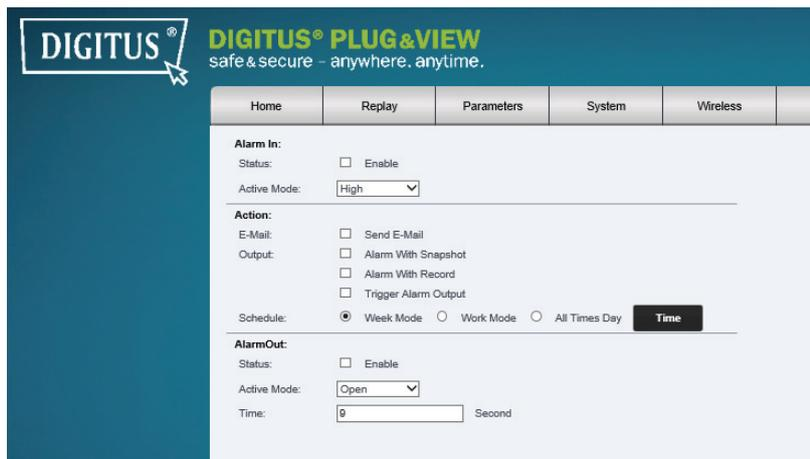
If your camera has “Alarm In and Out”, you can configure the settings here. You can use a sensor to trigger the alarm in. Please configure, if the used device will trigger the input with a high or a low signal.
