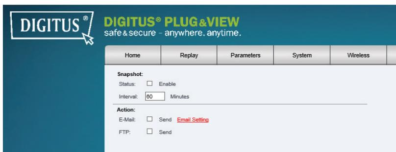
In Snapshot you can configure to take a snapshot in a specified interval. Please enable the status and configure the interval the snapshot should be taken. Choose as action if the snapshot should be send by e-mail or upload via FTP.
