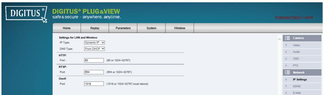
Here you assign a fixed IP address to the camera, according to the configuration of your LAN or WLAN, or select DHCP if you are using a DHCP-server, such as your router, for the assigning of IP-addresses. The ports for HTTP, RTSP and ONVIF can be modified here, if port forwarding settings are required on your router.
