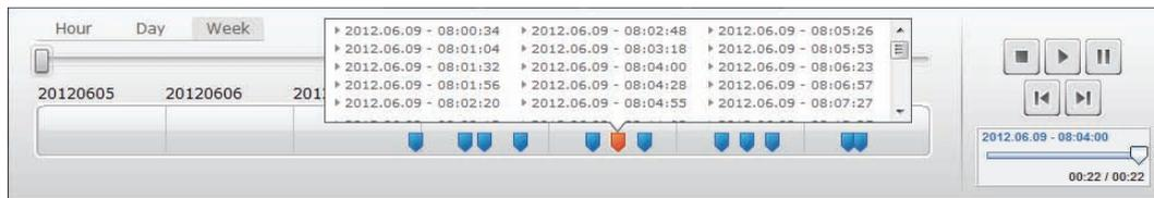
During playback of the selected media clip, you can stop or pause it, or switch to the next clip, using the **media control buttons**. You can also **drag the marker of the video search control** to the desired position in the playback.
