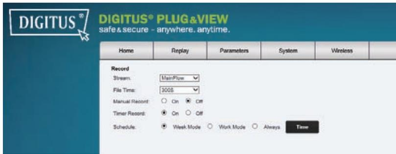
You can record the cameras stream to the installed SDCard. Please choose which stream you would like to record (MainFlow or MinorFlow) and configure the file size by using the file time. You can configure the file time from 30 seconds up to 600 seconds. Please choose if you want to do a manual record or if you want to do time recording. For time recording, you can configure the schedule for week mode, work mode or all time day.
