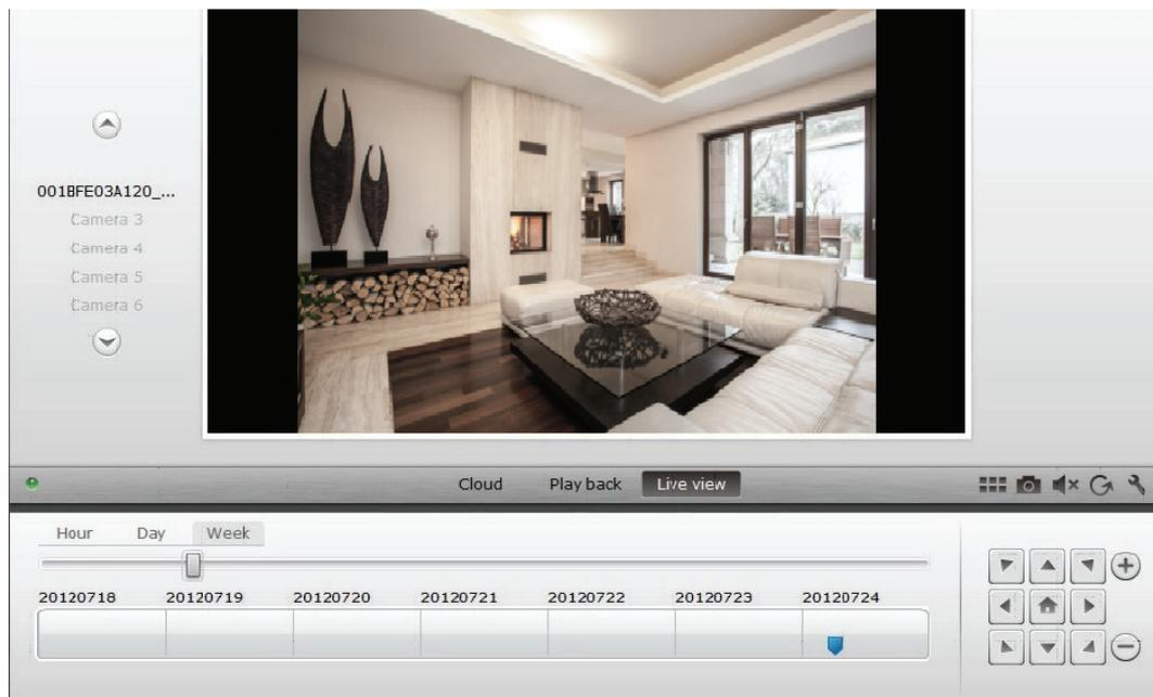
If the selected IP camera supports PTZ functions, the PTZ control panel, with which you can control the camera, can be selected. Otherwise the field will be grayed out to indicate that it has no function. Each motion adjustment requires a click.
