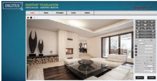
Under "Home" you can also pan and tilt (Plug&View OptiArc or similar PTZ cameras), as well as control the video settings such as brightness, contrast and saturation.
