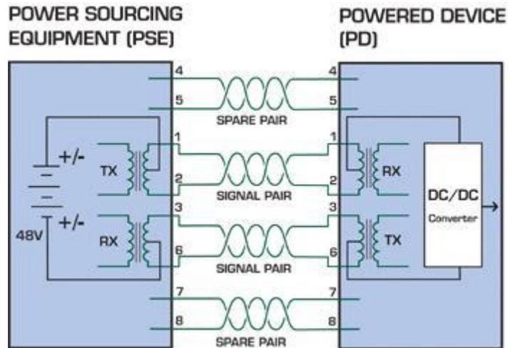
**Figure 5-1-2 - Power Supplied over the Data Pins**
