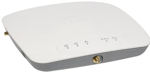
The NETGEAR ProSAFE® WAC730 is a high performance 3 x 3 business class dual band 802.11ac wireless Access Point (AP) that can support an aggregate throughput of up to 1.75Gbps (450Mbps for 2.4GHz and 1.3Gbps 802.11ac for 5 GHz). WAC730 operates in standalone or ensemble mode for centralized group management of up to 10 like Access Points without additional hardware, licenses or support fees. WAC720 is also WC7600/WC9500 Controller and Business Central cloud ready.
