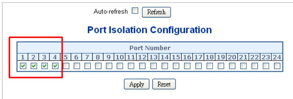
Figure 4-6-17: The Configuration of Isolated and Promiscuous Port
