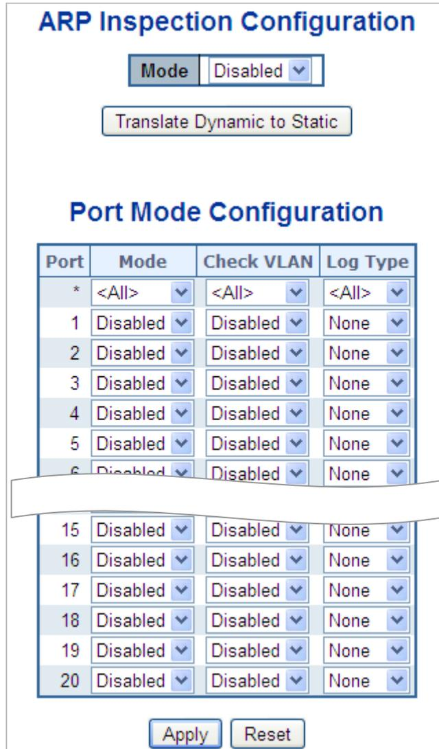
Figure 4-12-13: ARP Inspection Configuration Screen Page Screenshot
