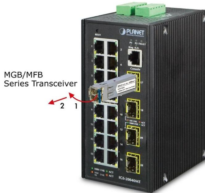
**Figure 2-10:** Pull out the SFP Transceiver Module
