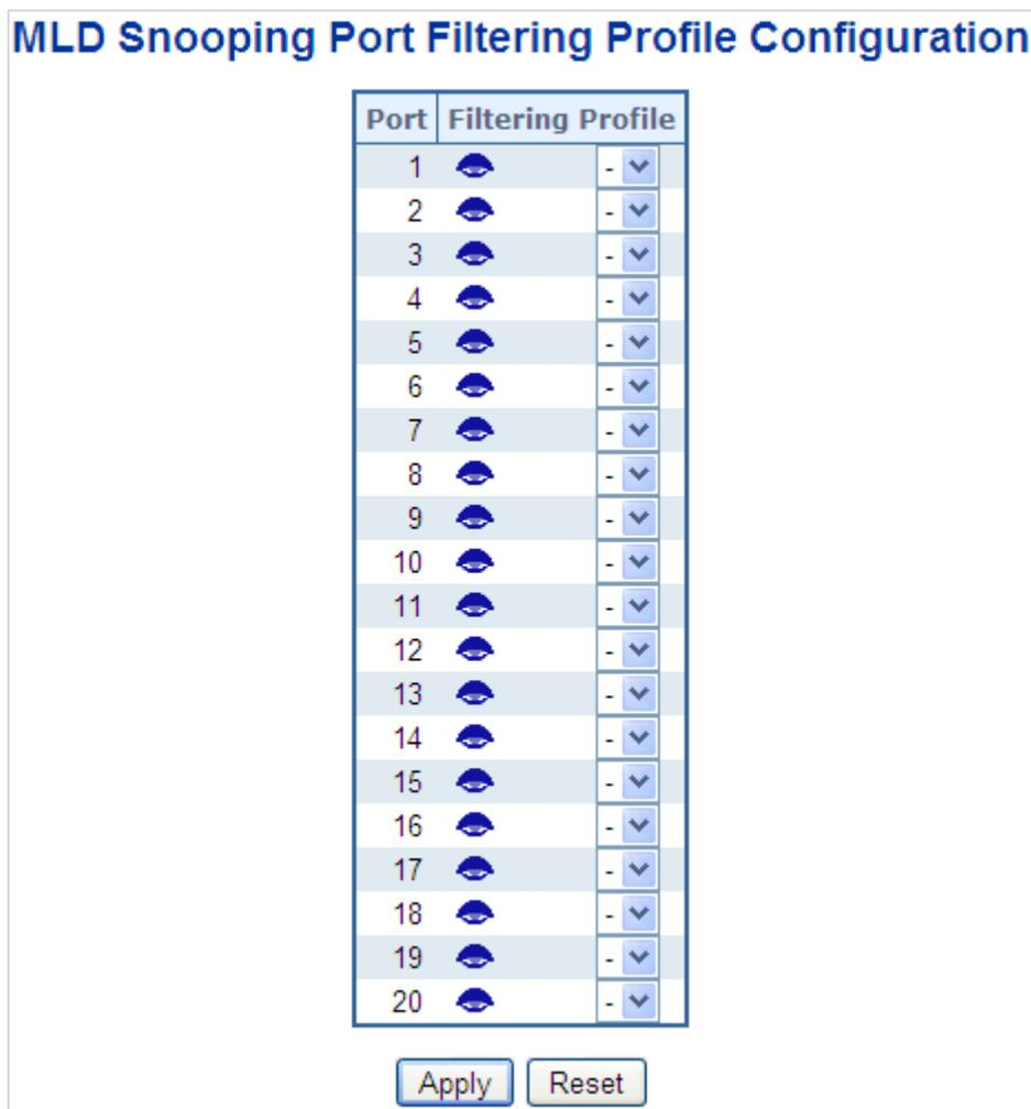
Figure 4-8-15: MLD Snooping Port Group Filtering Configuration Page Screenshot
