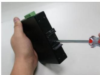
**Step 2:** Place the wall-mount plate on the rear panel of the Industrial Power over Ethernet Extender.
