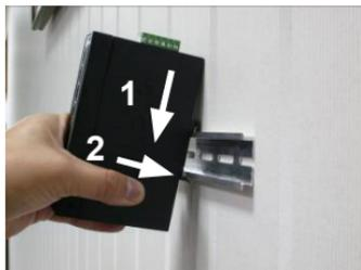
**Step 2:** Check if the DIN rail is tightly on the track.
