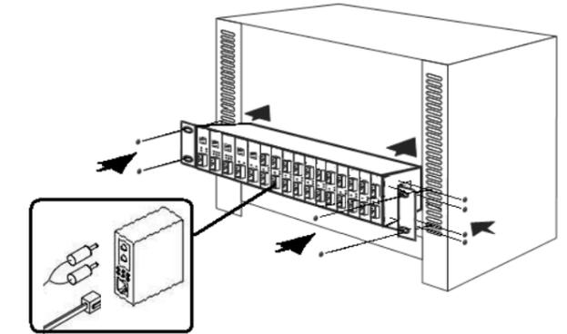
Figure 6-1 Installing Media Chassis in Wiring Closet Rails
