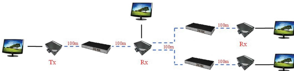
The more Network Switches, the longer distance extended. The number of Network Switches is as many as user want.
