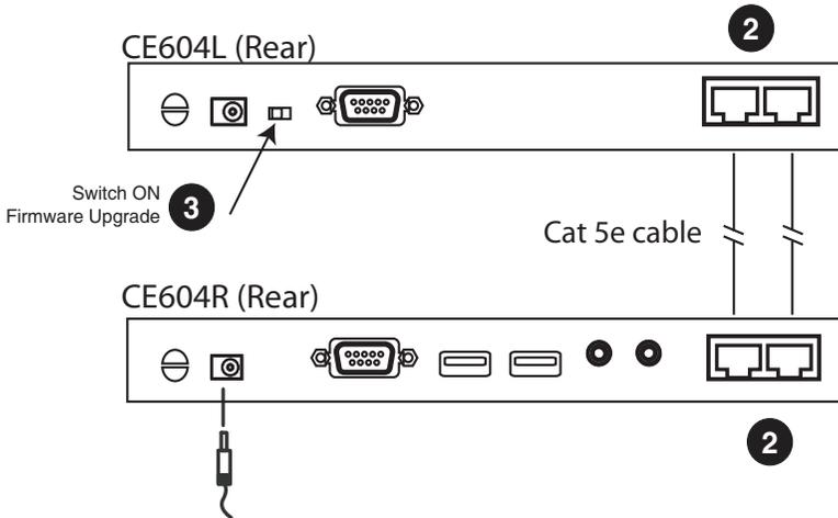
4. Plug in the power adapter and power on the CE604R.
