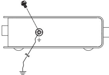
2. Make sure that the computer that the Local Unit connects to and the monitor that the Remote Unit connects to are properly grounded.
