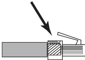
In either case, make sure that the sides of the RJ-45 connector make tight contact with the grounding contacts on the sides of the RJ-45 socket as shown in the diagram below:
