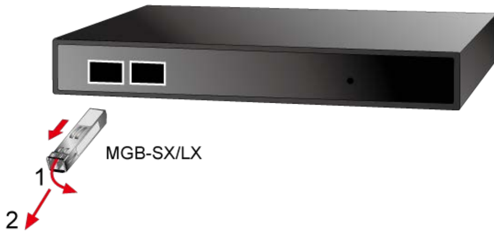
Figure 2-8 How to Pull Out the SFP Transceiver
