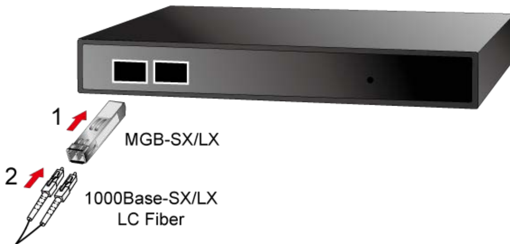
Figure 2-5 Plug in the SFP transceiver
