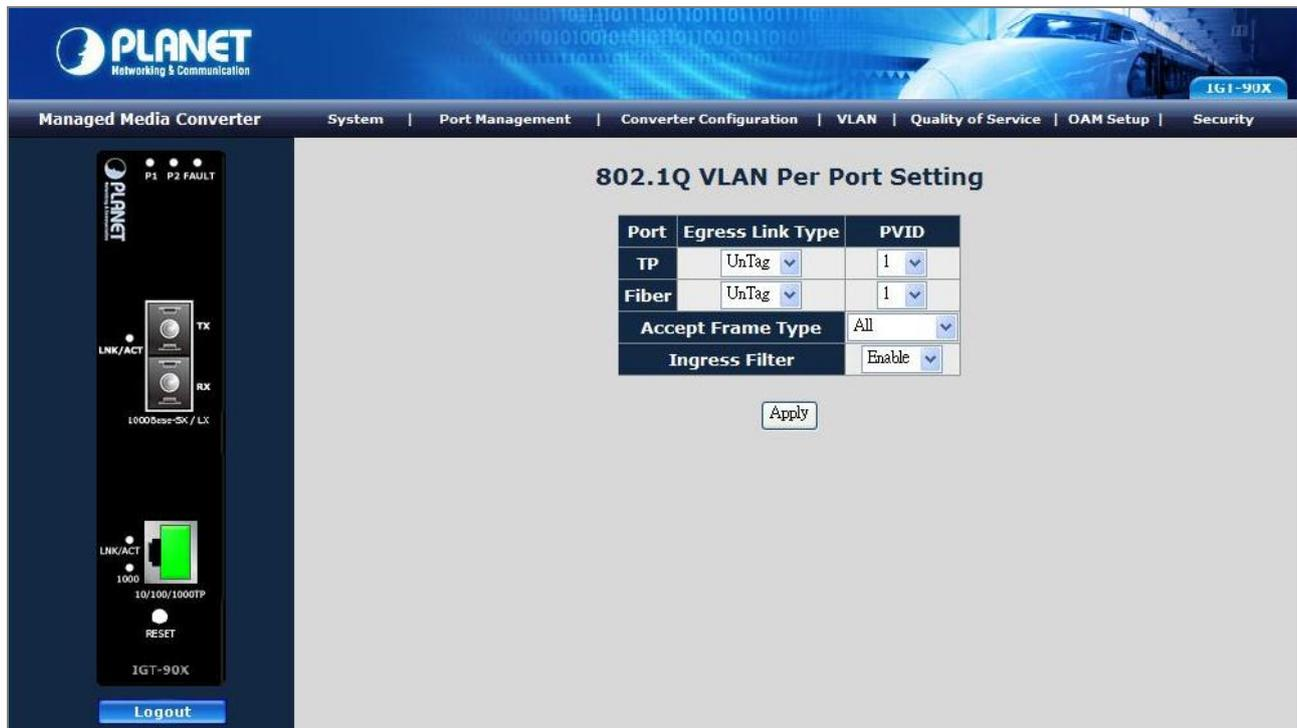
**Figure 4-28** VLAN Per Port Setting Web Page screen
