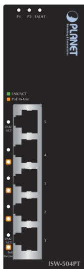
Figure 2-1 ISW-504PT front panel
